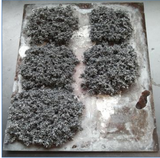
Figure 11: Intumescent coating C2, T2-2, T2-4, T2-6 and T2-8 after furnace test of 800°C
