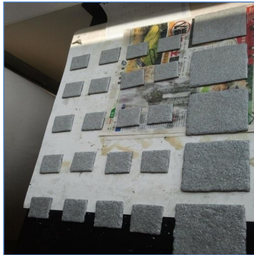
Figure 9: Intumescent coating (3mm) after fully cured
