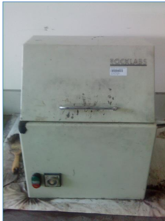
Figure 6: Rock Labs Grinder for grinding process
