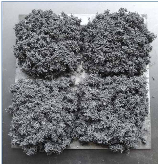
Figure 12: Intumescent coating F1-2, F1-4, F1-6 and F1-8 after furnace test of 800°C
