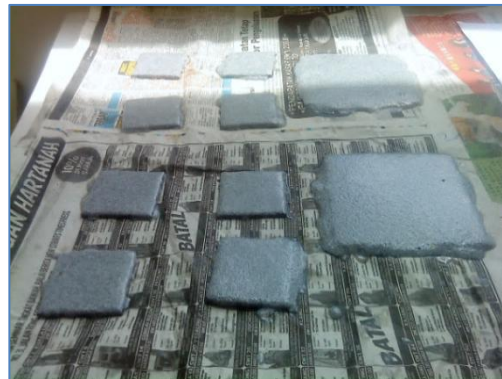
Figure 8: Picture of Intumescent Coating on the Curing Process
