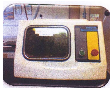
Figure 3.6 : Abrasive cutter (ferrous) at Block 17 used to cut the intended region
