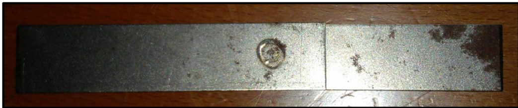
Figure 4.1 : Lap Shear Resistance Spot Weld specimen of Mild Steel sheet
