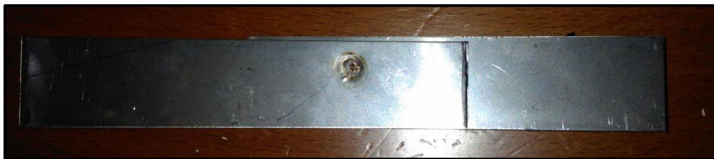
Figure 4.2 : Lap Shear Resistance Spot Weld specimen of Stainless Steel sheet
