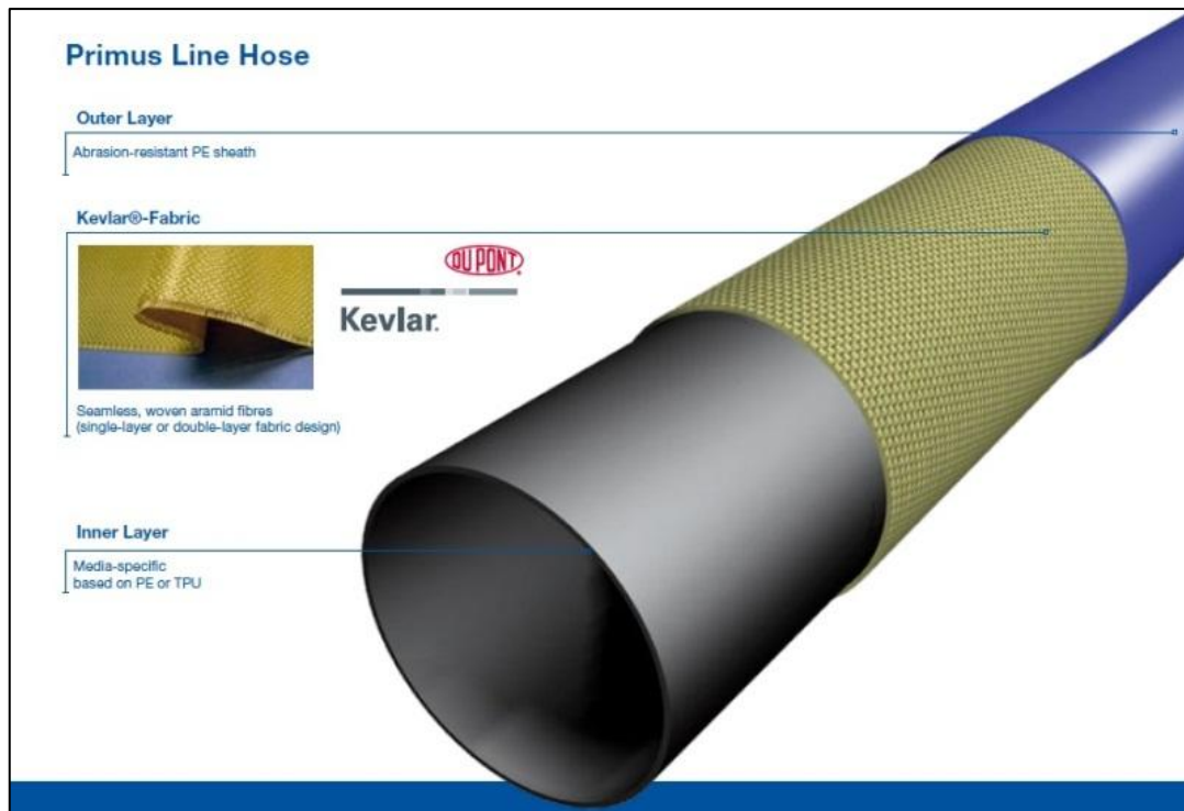
Figure 2.1: Schematic of Primus Line ® DN 200 PN 25 by layers.
