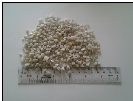
Figure 9 Bigger grains of silica sands collected from an area in Tronoh. Grains size ranging from 0.5mm to 0.3 mm
