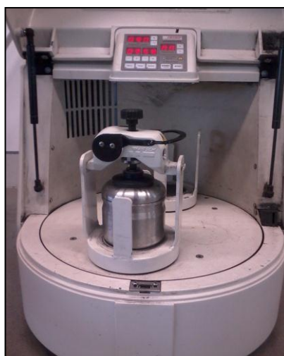
Figure 12. Planetary Low Energy Ball Milling machine
