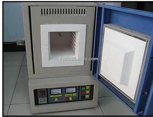
Figure 14. Furnace used for heat treating of SiC samples
