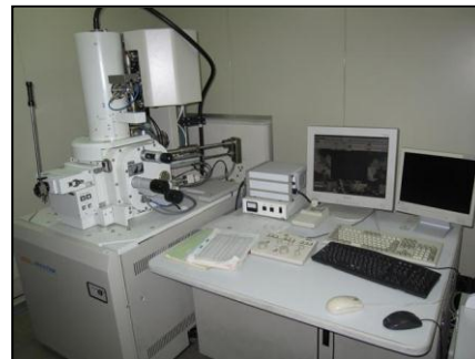
Figure 16 FESEM devices to carry the morphology of SiC
