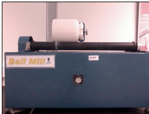
Figure 10 Low energy ball milling machine
