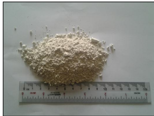
Figure 11 Average size of 30-63 \mu m silica powder after milling for 5 hours
