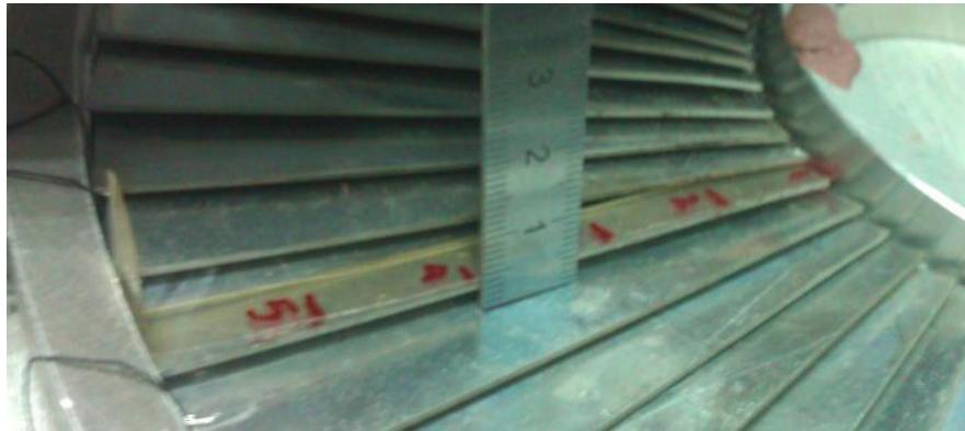
Figure 4.13 Gap Measurement between One Blade and Another at Point 1,2, and 3 of The Sampler
