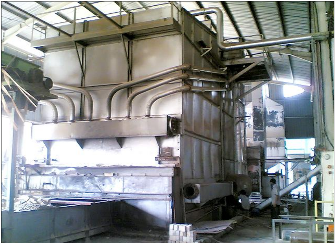
Figure 11: Yoshimine Water Tube Boiler
