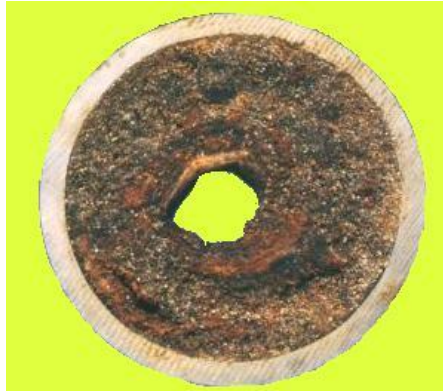
Figure 1-5: Wax formations reduced the interior diameter of a pipe (Source: PhillipsPetroleumCo.com)
