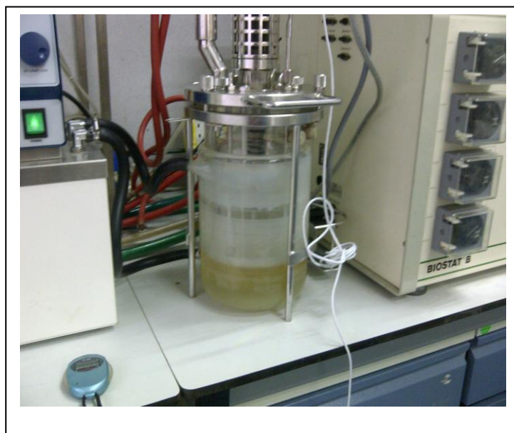
Figure 4.3: The melted stearic acid is added with DETA and the time required for the reaction is recorded using a stopwatch.
