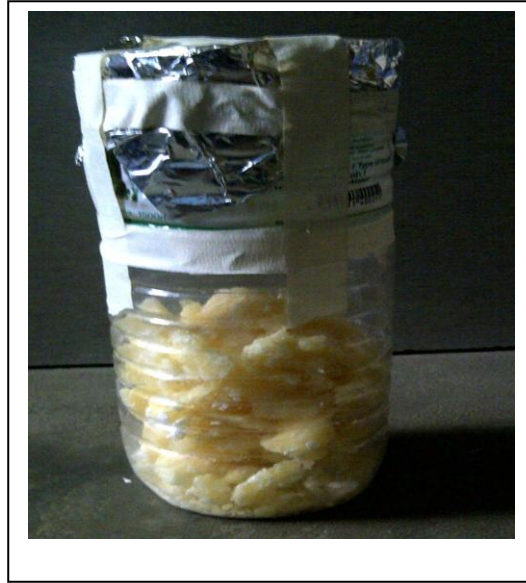
Figure 4.4: The mixture of Stearic acid and DETA solidifies as it cools down to room temperature (23-24 degrees Celcius)
