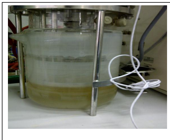
Figure 4.2: The Stearic Acid is heated with the reactor at 100 degrees celcius and forms a viscous solution
