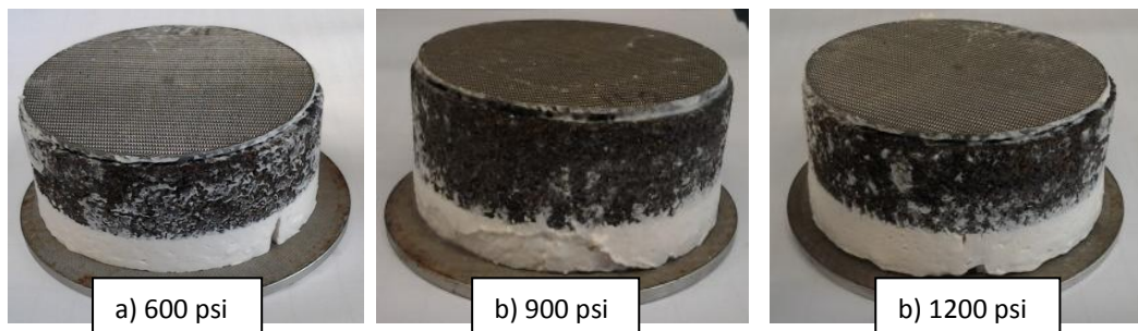
Figure 4.9 – 15% of resin coated with different pressure in gravel packing application.
