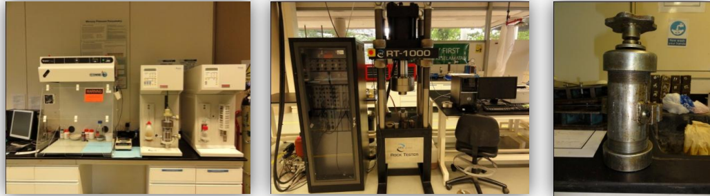
Figure 3.2 – Tools Required (Porosimeter, Compression Test, and Mould). Taken from UTP laboratory at block 14.
