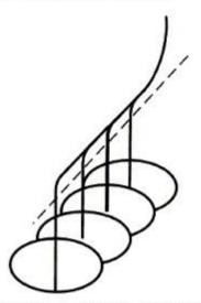
c) Multibranch well with fractured vertical branches (horizontal parent well is drilled above the reservoir).
