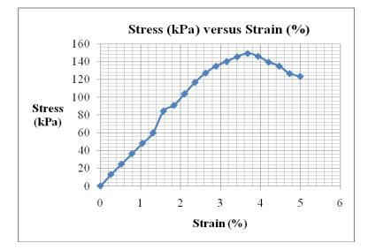
Figure 4.2.0: Stress (kpa) versus strain (%) of peat specimen mixed with 14% lime & cured for 14 days.
