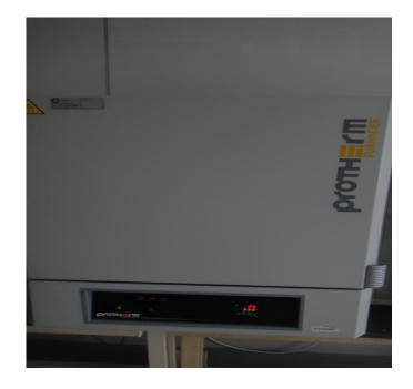
Figure 3.3.4: Muffle Furnace for determinating peat organic content
