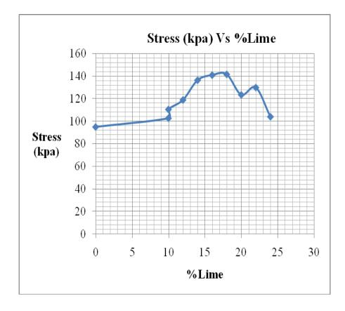
Figure 4.2.1: Stress (kpa) versus lime (%) of peat specimen mixed with 0%, 10% to 24% lime & cured for 0 & 7 days
