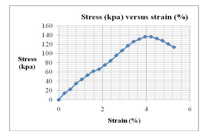
Figure 4.1.9: Stress (kpa) versus strain (%) of peat specimen mixed with 14% lime & cured for 7 days.
