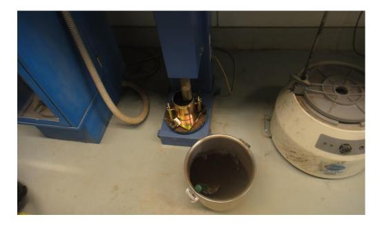
Figure 3.3.8: Standard proctor test
