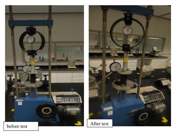
Figure 3.4.0: Unconfined compression test (UCT)
