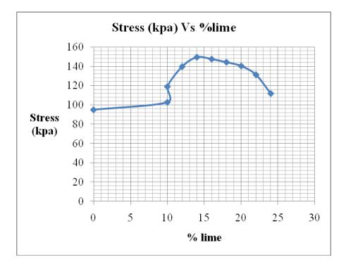
Figure 4.2.2: Stress (kpa) versus lime (%) of peat specimen mixed with 0%, 10% to 24% lime & cured for 0 & 14 days.
