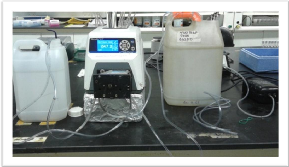
Figure 3.7: Sequencing Batch Reactor run-up test for with tap water to ensure efficiency before running with sample.
