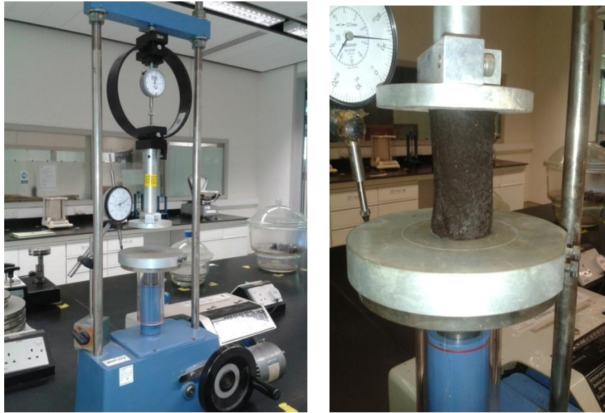
Figure 2.5: Unconfined Compressive Strength Test
