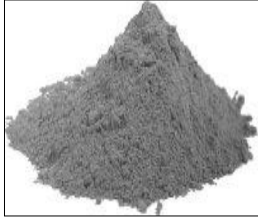
Figure 2.4: Ordinary Portland Cement
