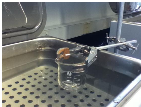
Figure 3. 4 : The methanol solution is kept in the water bath until it reach the desired temperature
