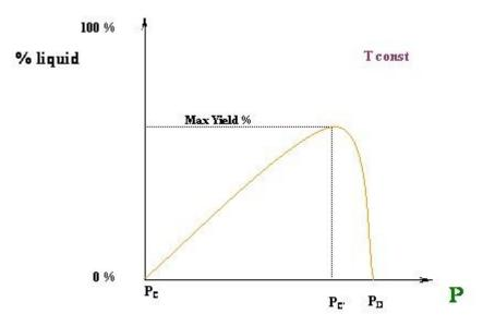
Figure 2.2: Liquid Yield for the Isothermal Compression
