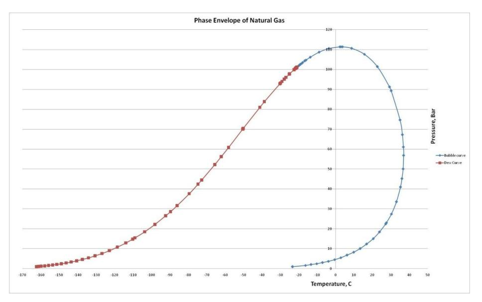
Figure 4.1: Phase envelope of natural gas simulation
