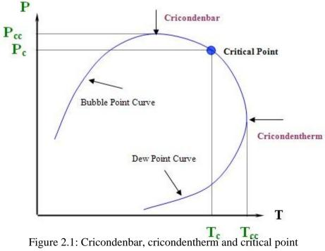
From phase diagram on figure 2, cricondenbar point to cricondentherm point call as retrograde curve. Cricondenbar is the point where pressure point of vapor-liquid coexistence for multi-component system. For cricondentherm, this point is where the temperature point of vapor-liquid coexistence. This two point same as for single component system that is bubble point and dew point.
