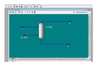
Figure 3.1: Process flow diagram for condensation of natural gas
