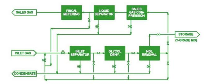
Figure 1.1: Example of process flow diagram for natural gas liquids recovery plant
