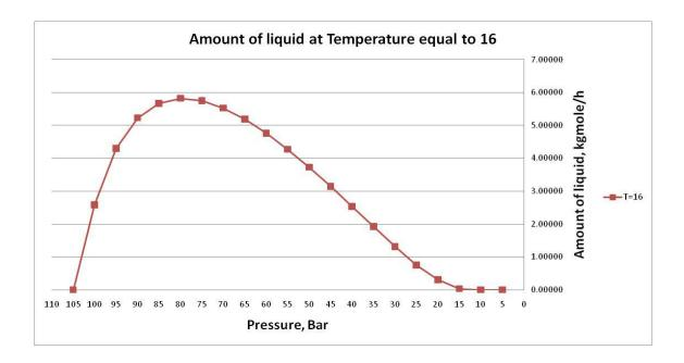
Figure 4.2: Amount of liquid drop form at temperature equal to 16°C
