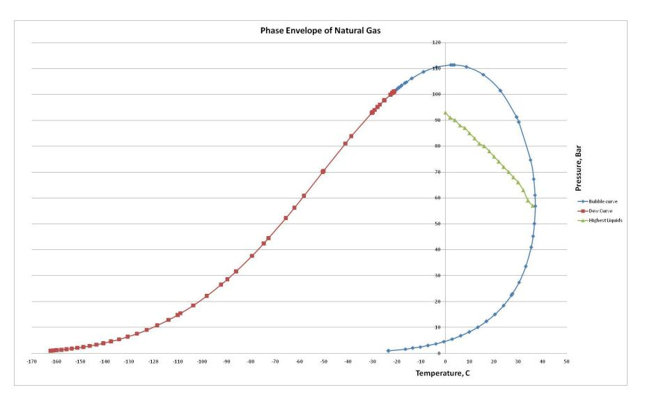
Figure 4.3: Highest liquid drop curve in phase diagram
