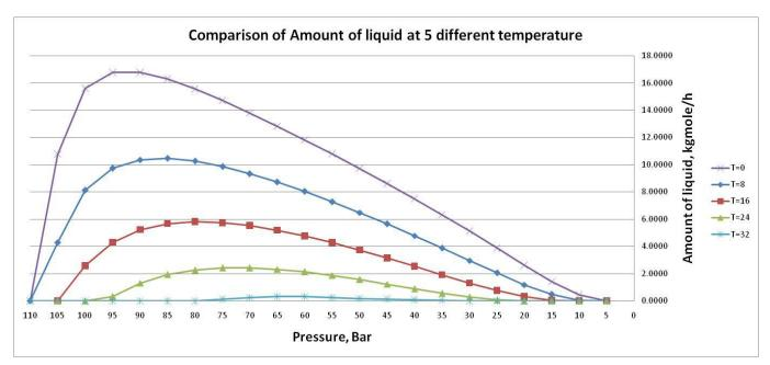
Figure 4.4: Comparison of liquid drop formation at 5 different temperatures
