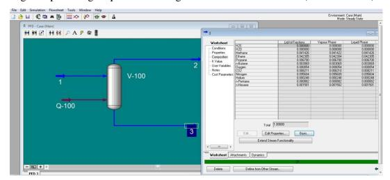
Figure 3.2: Example of liquid percentage detail after separation using flash drum
