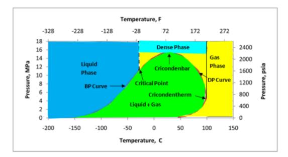
Figure 2.3: Dense phase for typical natural gas phase diagram
