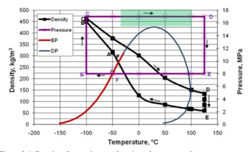
Figure 2.4: Density of natural gas as function of pressure and temperature
