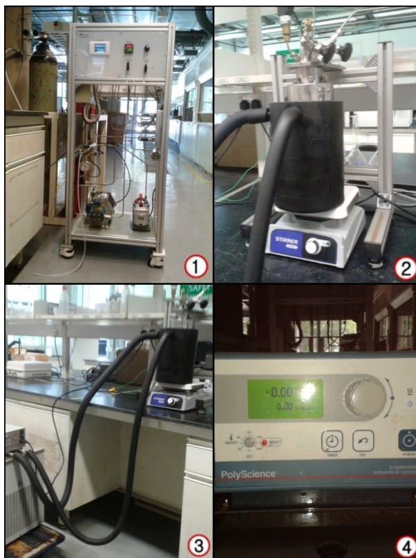
Figure 3.3.1: The Equipment used for Part I and Part II Experiment. 1:Gas Mixing Equipment, 2:Reactor that immersed in the water bath, 3:Circulation of water bath for rapid increase of temperature, 4:Programmable Temperature Controller
