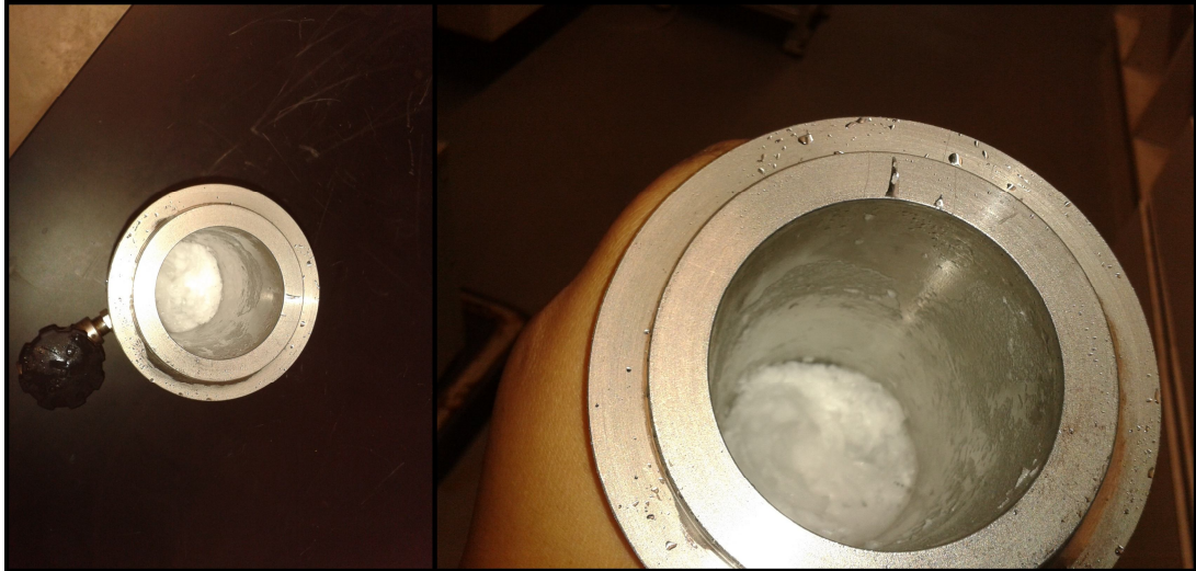
Figure 5.2.1: Gas hydrate of mixed \text{CO}_2\text{-CH}_4
