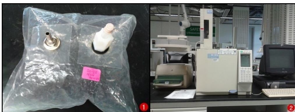
Figure 4.2.1.1 : 1) Sample collected in the tedlar sampling bag. 2) Gas Chromatography
