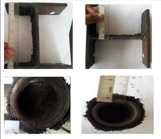
Figure 7 : Char Expansion Measurement Method for I-Beam, T-Joints, Pipes and Elbows
