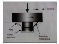
Figure 8 : FSP tool diagram
