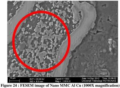
The darker colour region in the image shows the Aluminum and the less dark colour region in the image is Copper. The Nano Metal Matrix Composite of Aluminium Copper formed at the region marked in the figure 24.
