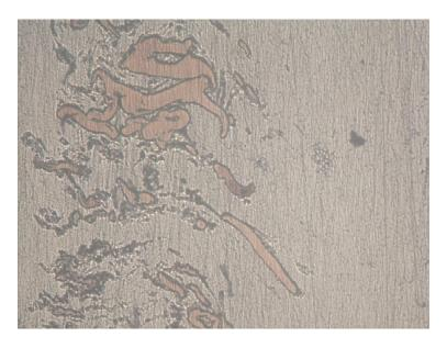
Figure 19 : Microstructure image of MMC surface with 10X magnification
