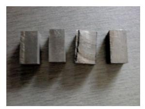
Figure 15 : Nano Metal Matrix Composite after been cut
