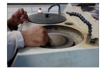
Figure 18 : Polishing process
