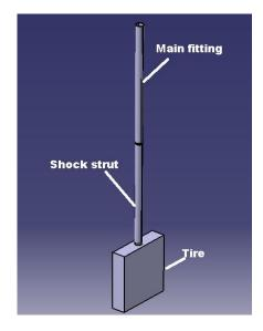
Figure 3-5: Simplified model with separated bodies
