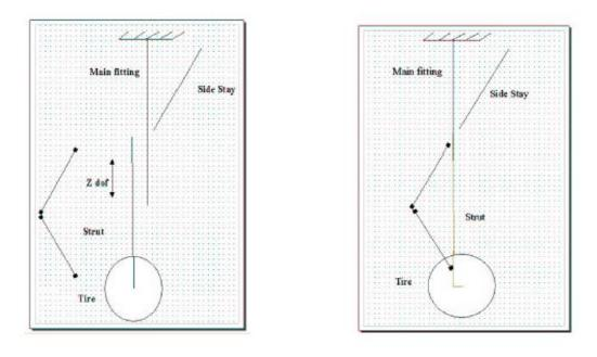
Figure 2-2: Proper landing gear model for the modal analysis [4]
