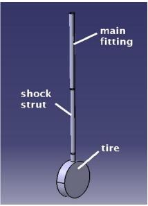
Figure 3-6: Modified model of the landing gear
