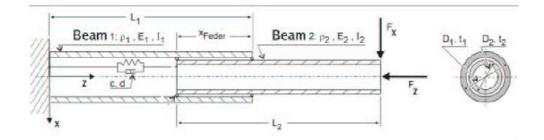
Figure 2-1: Landing gear in the form of beam model [4]
