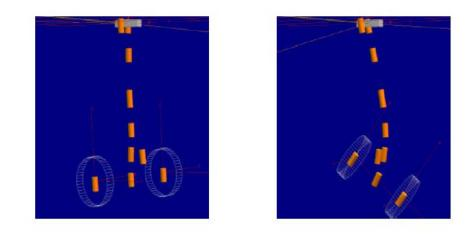
Figure 4-7: Mode shape of a landing gear [7]
