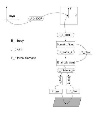
Figure 3-2: Schematic diagram of the landing gear [7]
