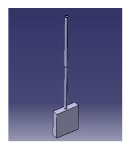
Figure 3-4: Simplified model of the landing gear
