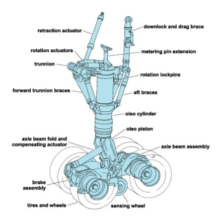
Figure 1-1: Components of a landing gear [1]
