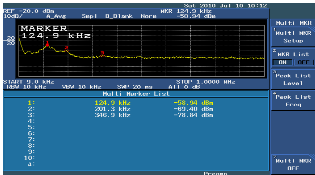
Figure 21: Example of frequency spectrum representation in Spectrum analyser displayer
