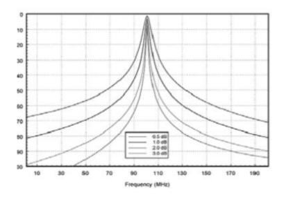
Figure 3: Shows insertion loss characteristics
