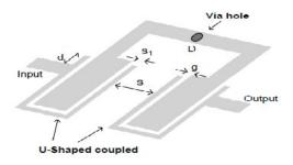
Figure 5: Structure of a quarter-wavelength SIRs bandpass filter.
