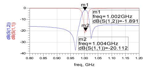
Figure 16: Simulated Quasi elliptic dual mode filter
