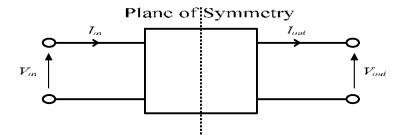
Figure 2: Symmetrical two-port network
