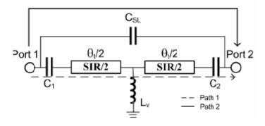
Figure 6: Equivalent circuit of a quarter-wave SIRs bandpass filter.
