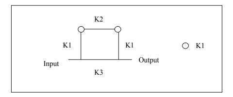
Figure 12: Coupling and routing structure filter design
