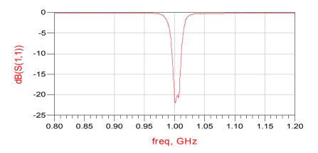
Figure 18: Reflection Coefficient in Microstrip
