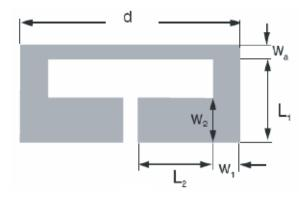
Figure 9: Proposed folded stepped impedance resonator
