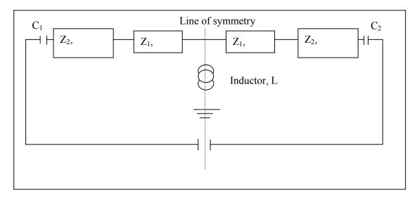
Figure 11: Filter design topology
