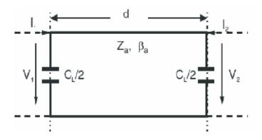
Figure 8: Equivalent circuit of proposed stepped impedance resonator
