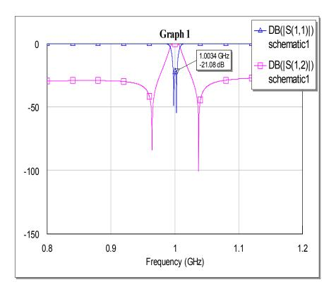
Figure 13: Simulated quasi-elliptic filter response
