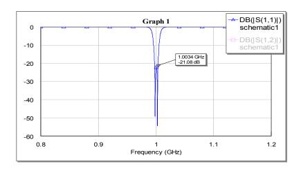
Figure 15: Reflection coefficient response
