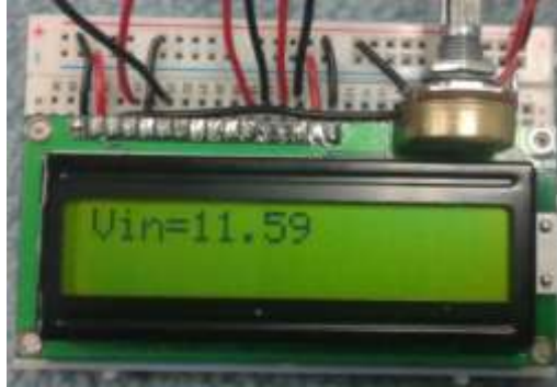
Figure 14 : 16x2 Liquid Crystal Display
