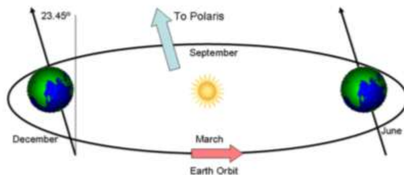
Figure 3 : Inclination and rotational of Earth that affect the PV electricity generation system[5]
