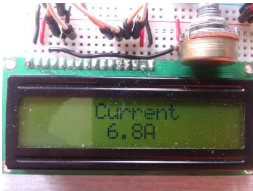
Figure 19 : Display Current of the Battery
