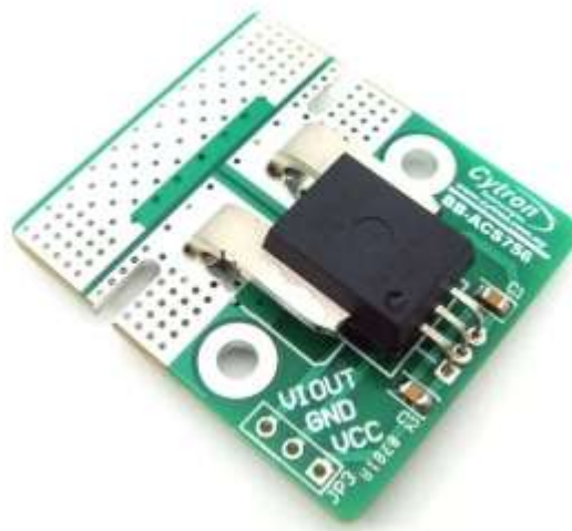
Figure 12 : BB ACS 756 current sensor
