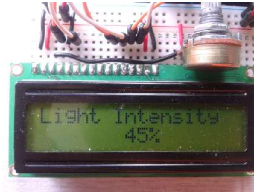
Figure 22 : Display Light Intensity Surrounding the Battery
