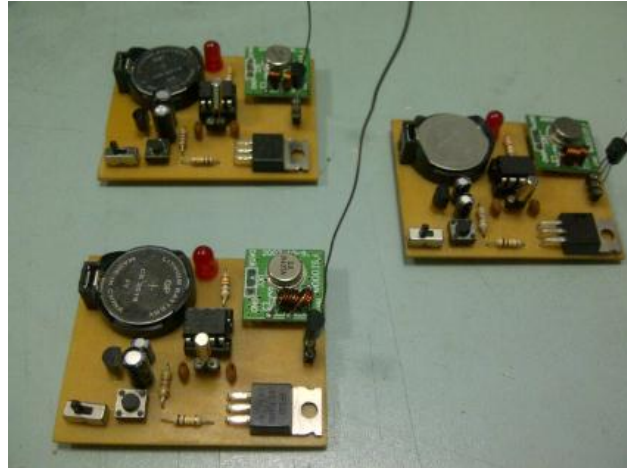
FIGURE 43. Final Prototype of Sensor Nodes Developed into PCB
