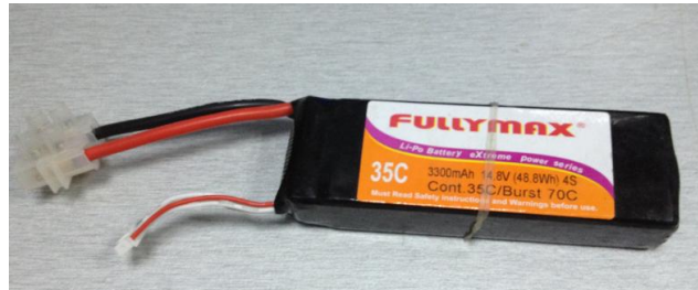
Figure 34: FullyMax 14.8V 3300mAh 4S 35C LIPO
