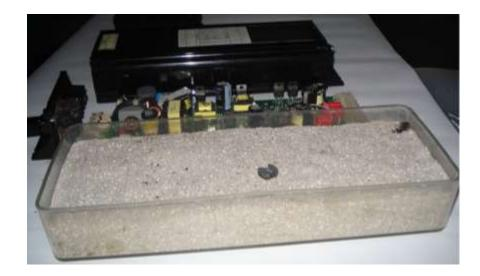
Figure 15: Sand inside the ballast casing
