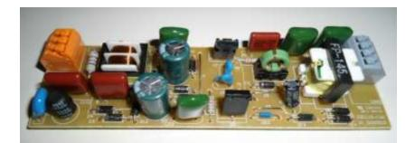
Figure 9 : Electronic ballast circuitry [13]
