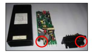
Figure 2 : Damaged electronic ballast which is used in salty environment (offshore) at Petronas Carigali, Miri, Sarawak
