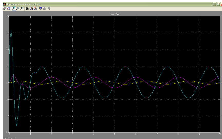
Figure 4.2-2: Acceleration (a1), velocity (v1) and displacement (x1) graph of unsprung mass (m1) scope for sine input for 3 DOF (with driver)
