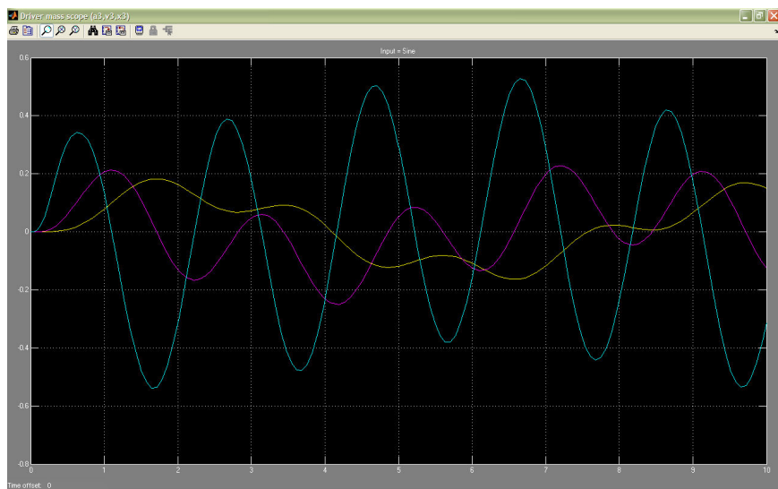
Figure 4.2-4: Acceleration ( a_3 ), velocity ( v_3 ) and displacement ( x_3 ) graph of driver mass ( m_3 ) scope for sine input for 3 DOF (with driver)
