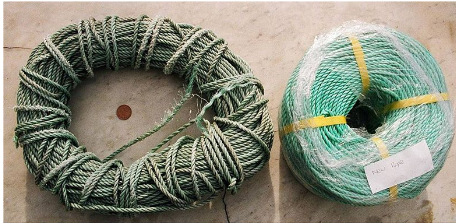
Figure 2.2: Effect of photodegradation on polypropylene rope
