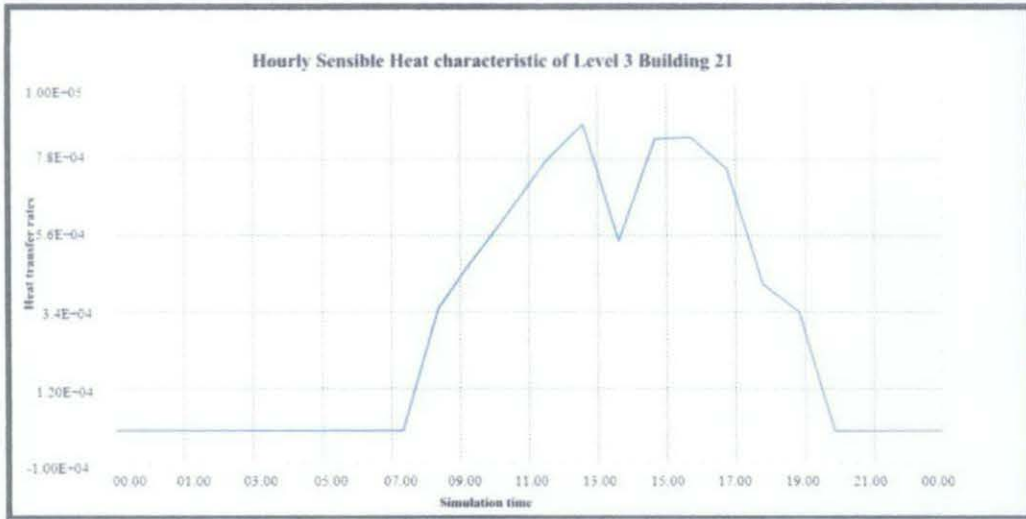
Figure 4.2: Sensible Heat characteristic of Level 3 Building 21
