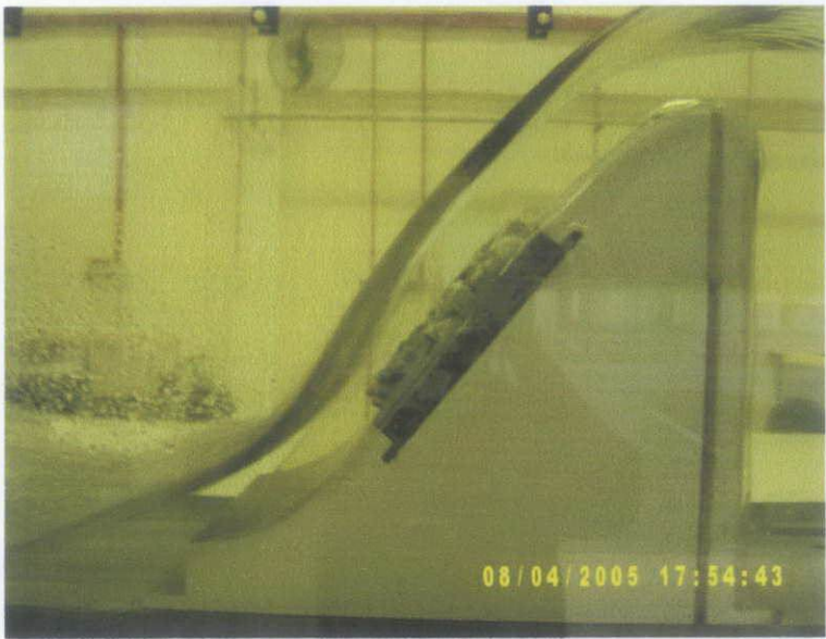
Figure 38: Side view if Design Model 2 at 80 m 3 /hr
