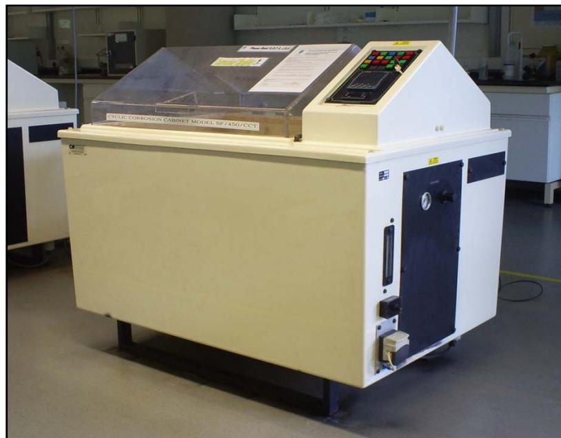
**Figure 3.2: Cyclic Corrosion Cabinet Model SF/450/CCT**
