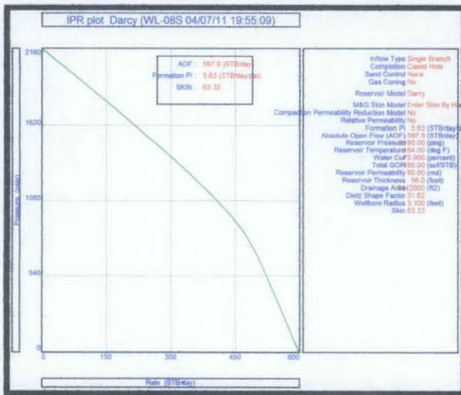
Figure 23: IPR plot for pre-acid WL-08S well model
