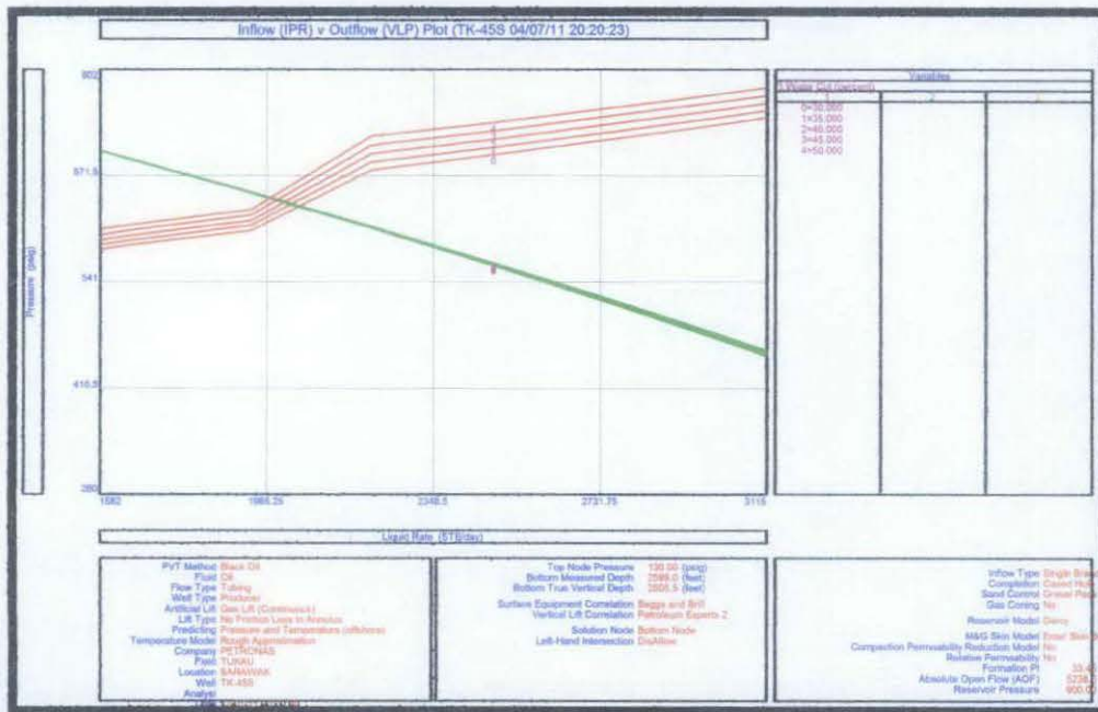
Figure42: Inflow versus Outflow plot with WC sensitivities for TK-455
