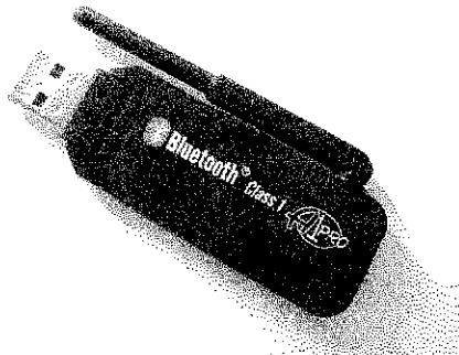
Figure 3.23: A USB Bluetooth dongle with antenna (100 m/378 ft range)
