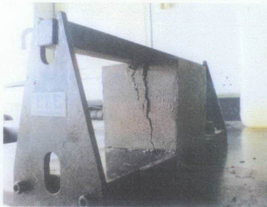
Figure 6. Placement of the concrete cube in the casing for Split Tensile test.
