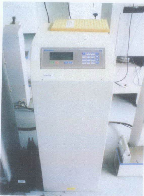
Figure 5a. Flexural and Compression Machine for split tensile test.
