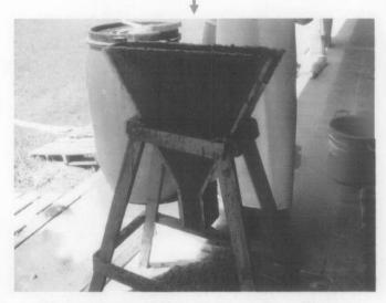
Concrete was falling free out of the funnel Figure 7: V-Funnel Test Process
