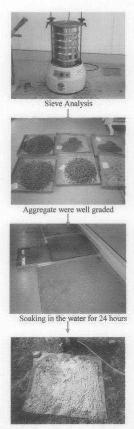
Rinse the aggregate before letting it dry at room temperature for another 24 hours Figure 1: Aggregate Preparation
