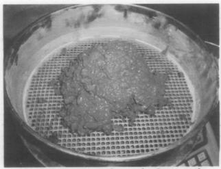
Concrete was poured onto the 5mm mesh
