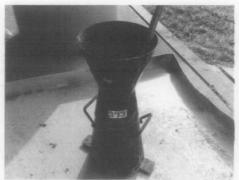
The truncated cone for slump flow test
