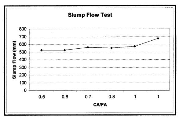
Figure 13: Slump Flow Test Evaluation
