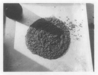
Figure 8: Slump flow without segregation
