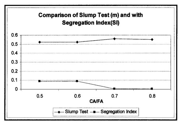
Figure 18: Comparison of result between Slump Test and Segregation Index (SI)
