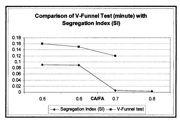
Figure 19: Comparison of result between V-Funnel Test and Segregation Index (SI)
