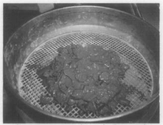
Concrete was poured onto the 5mm mesh
