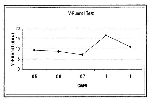
Figure 14: V-Funnel Test Evaluation
