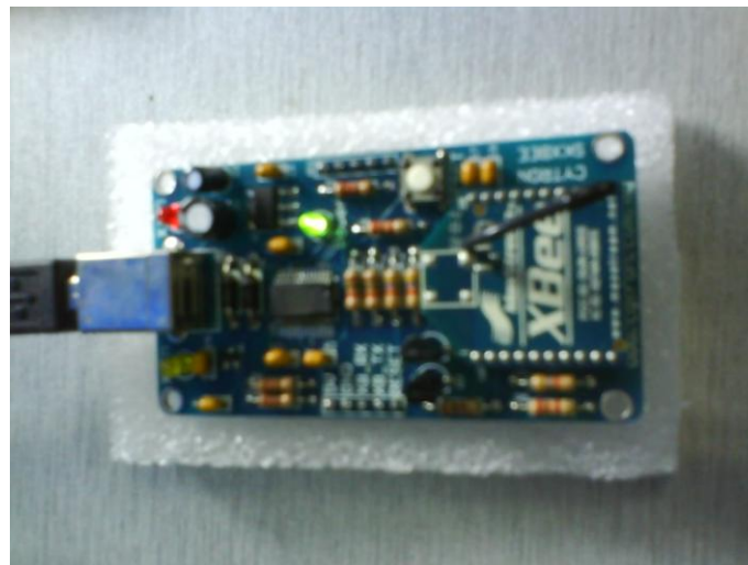
Figure 33 : SKXbee at PC system
