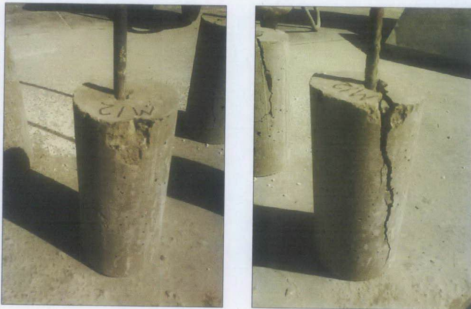
Figure 4.4 : Difference in physical appearance between round bar (picture : left) and ribbed bar (picture : right) after pull out test
