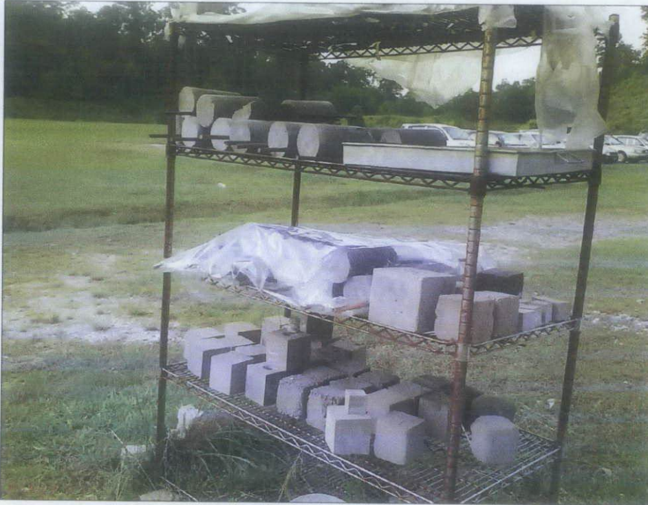
Figure 3.5: External exposure curing
