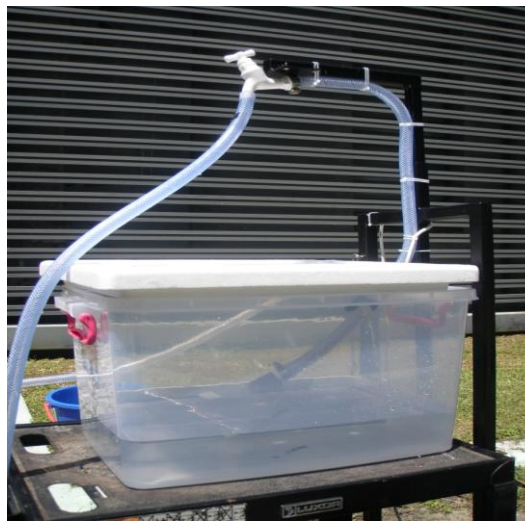
Figure 12: Pump with water container and control valve (head pipe)
