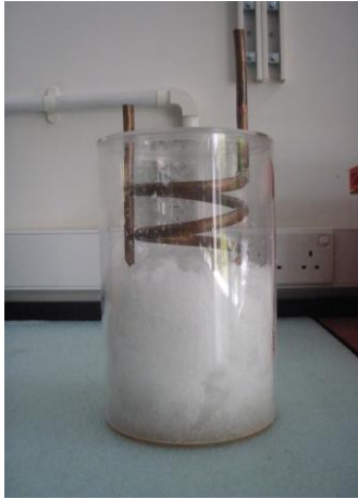
Figure 20: TES tank with PCM before testing
