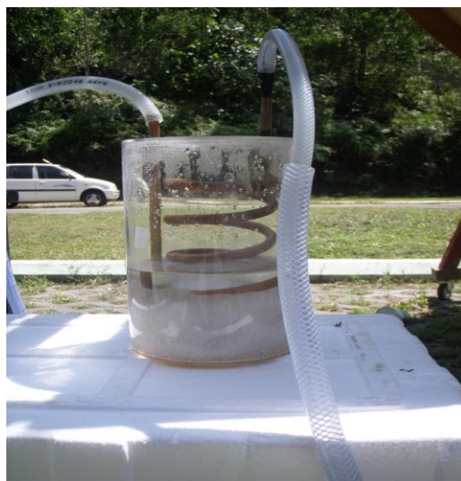
Figure 13: The TES tank during the experiment
