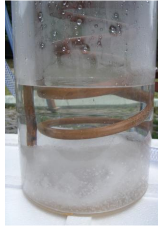
Figure 21: TES tank condition at 30°C (Phase change of PCM during the experiment)
