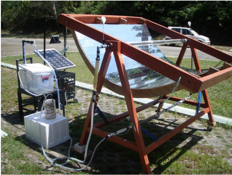
Figure 9: Experiment set-up during testing (Charging process)
