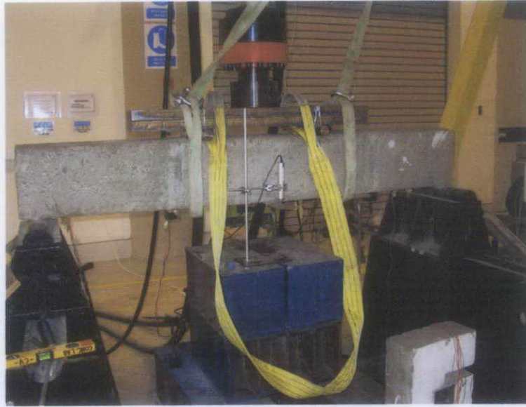
Beam was set up for dynamic test
