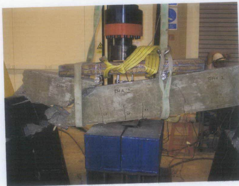
Failure for RHA 2 beam caused of movement of support
