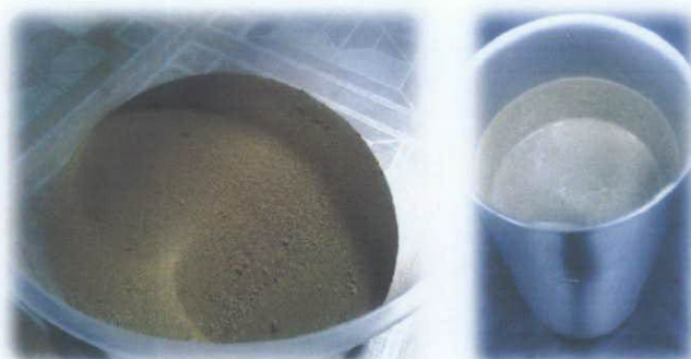
Figure 30. Coconut coir before mixing (left) and after mixed with drilling fluid (right)
