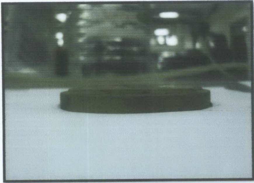
Figure 22 : Mud cake of B1 mud on 35 micron ceramic disk
