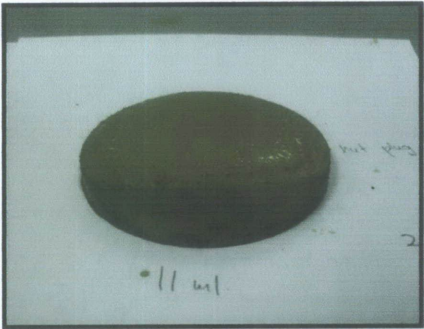
Figure 24: Mud cake of NP1 mud on 35 micron ceramic disk
