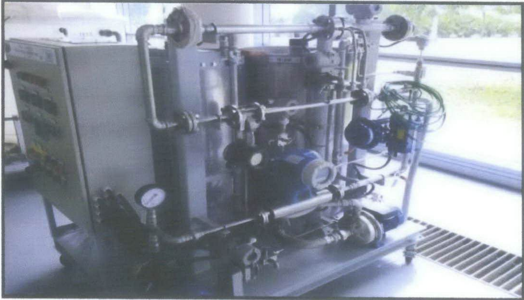
Figure 1 : PcA SimExpert Mobile Pilot Plant SE231B-21 Flow Control & Calibration Process Unit
