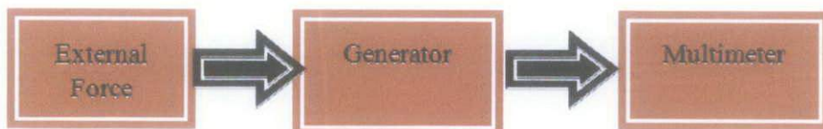
Figure 41: Test setup for open circuit test
