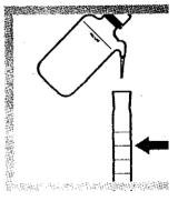
4. Blank Preparation: Fill a 25-mL mixing graduated cylinder to the 25-mL mark with deionized water.
