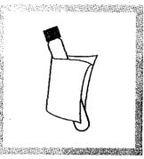
**10.** Wipe the outside of the vial with a damp cloth followed by a dry one, to remove fingerprints or other marks.
