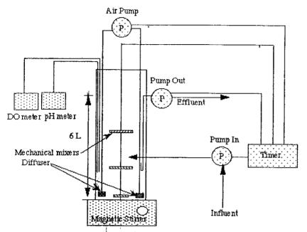
Figure 16. A typical SBR configuration.
