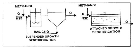
Figure 3: Separate Stage Nitrogen Removal System (Sedlak, 1991)
