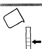
**Prepared Sample:** 3. Fill a 25-mL mixing graduated cylinder to the 25-mL mark with sample."
