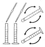
7. Pipet 1.0 mL of Nessler Reagent into each cylinder. Stopper and invert several times to mix.
