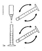
dd three drops heral Stabilizer to cylinder. Stopper and several times to mix.
