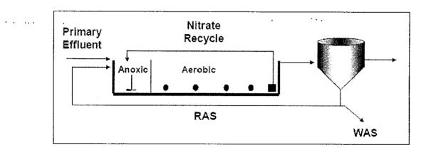
Figure 6: Layout of UTP's Anoxic Zone
