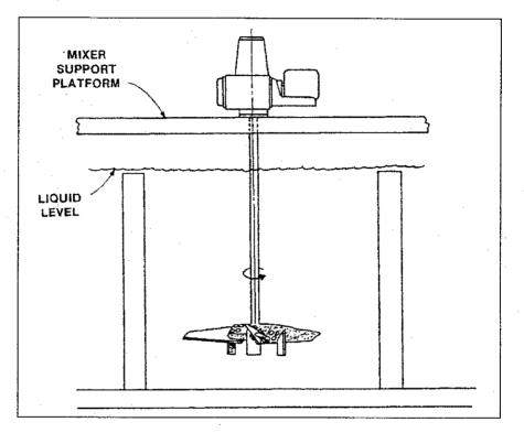
Figure 7: Typical Submerged Turbine Mixer
