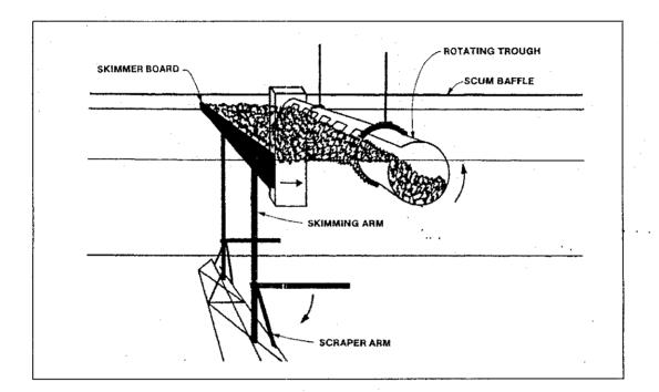
**Figure 8: Typical Rotating Skimmer Device**
