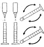
6. Add three drops of Polyvinyl Alcohol Dispersing Agent to each cylinder. Stopper and invert several times to mix.
