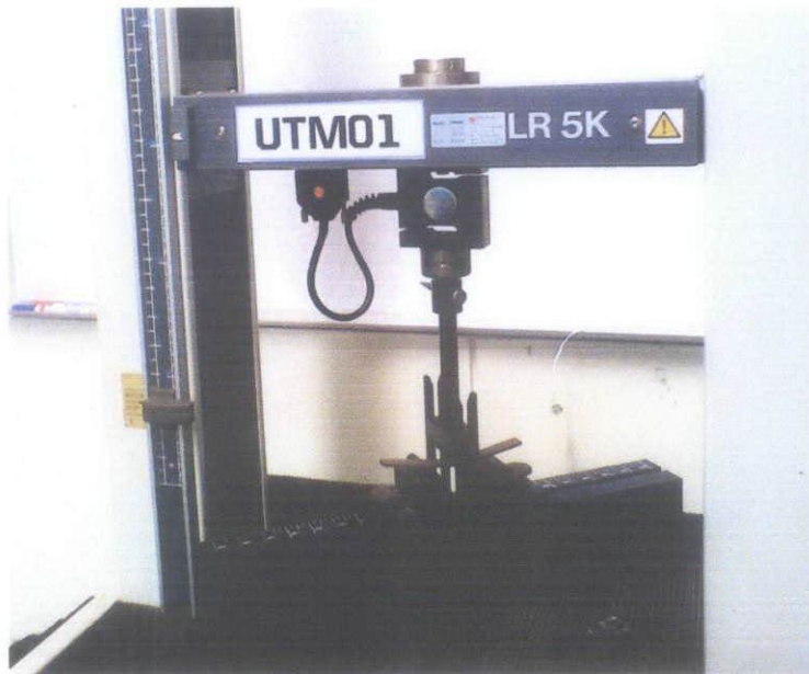
Figure 3.7: Flexural testing of the specimens at the lab using Universal Testing Machine.
