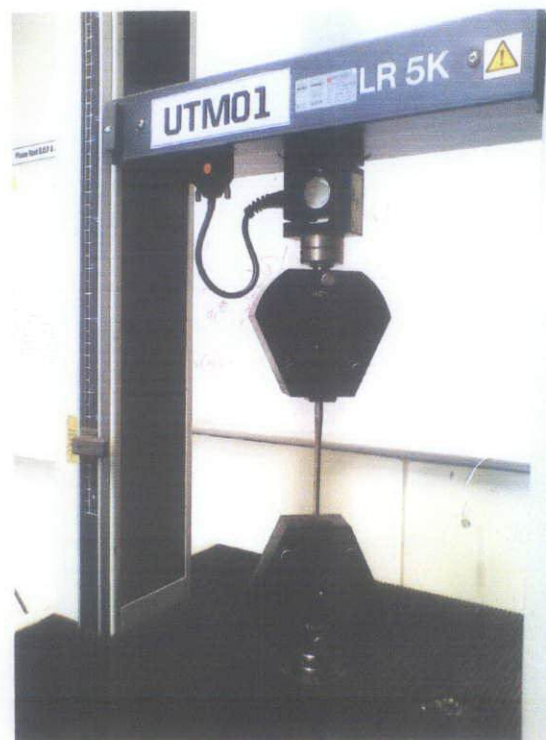
Figure 3.6: Tensile testing of the specimens at the lab using Universal Testing Machine.
