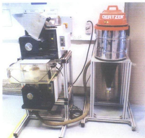
Figure 3.8: Lab Scale Grinder with particles size >500 \mu\text{m} .
