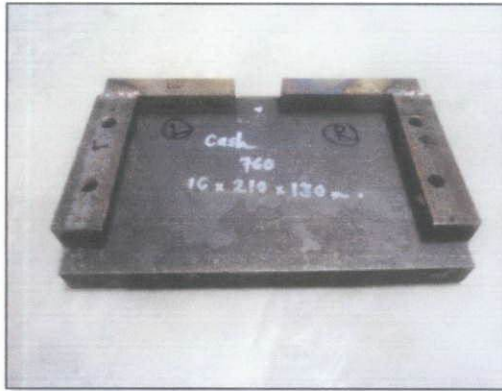
Figure 13: Aluminum plates will butt closely on jig and tightened with bolts and nuts
