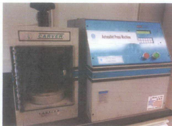
Figure 35: Carver Press Number 3887 Autopallet press machine.
