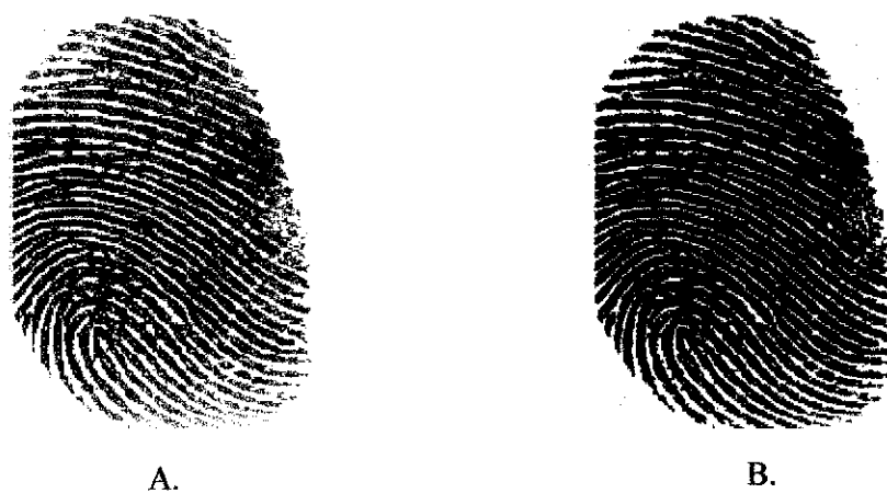
Figure 2.8: Fingerprint obtained after preprocessing: (A.) Original image, (B.) Enhanced image
