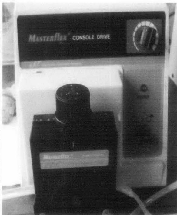
Figure A4: Pump for flow rate control
