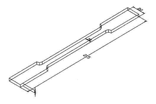
Figure D4: The dog bone-shaped specimen dimension in millimeter unit.
