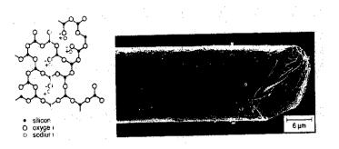
Fig. 4.62: G ass fiber let: molecular model richt: SEM photograph
