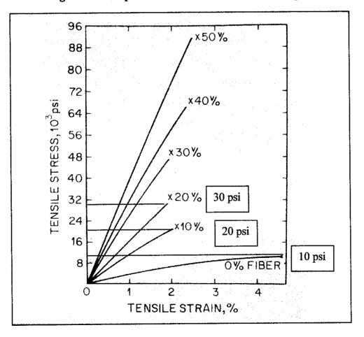
Figure 4.4: Theoretical value of tensile strength of typical fiber reinforced
