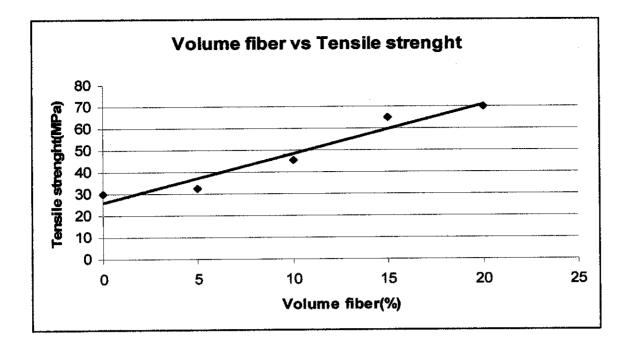
Figure 4.3: Graph of Volume fiber vs Tensile strength
