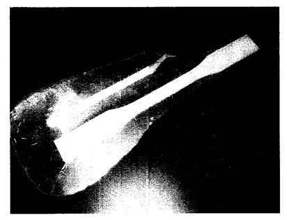
Figure D3: Molded Fiber reinforced using polypropylene and 5% of volume fiber
