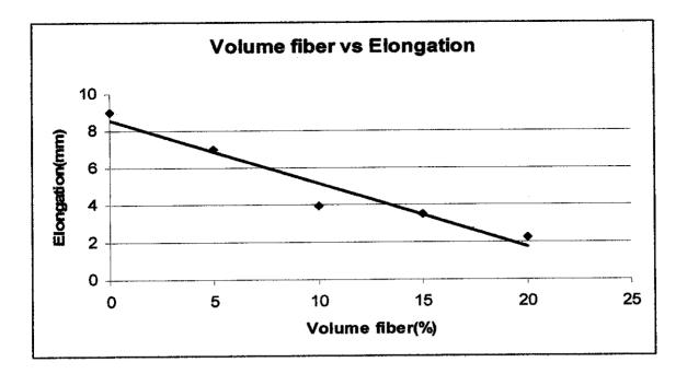
Figure 4.1: Graph of Volume fraction of fiber vs Elongation
