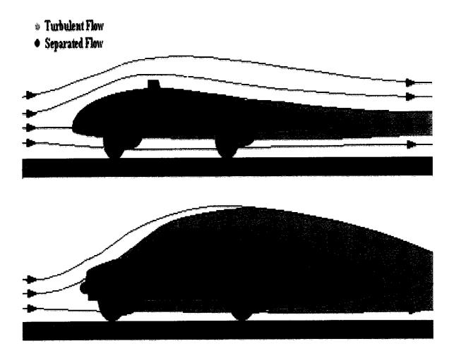
Comparison of conventional and aerodynamic car that can cause different set of wind flow upon the surface due to the design structure.
