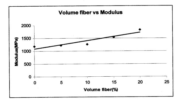
Figure 4.2: Graph of Volume fraction of fiber vs Young Modulus
