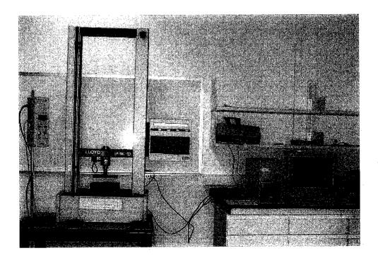
Figure 3.16: Universal Testing Machine manufactured by LLOYD Instruments, Germany
