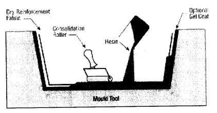
Fig 2.3: Schematic of the hand lay-up process
