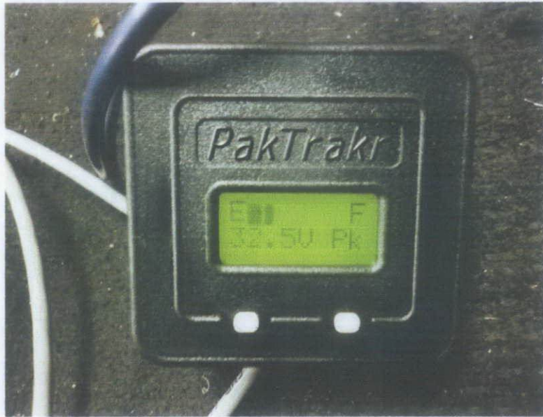
Figure 17 : PakTrakr displaying pack voltage
